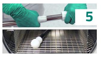
Loosen the telescopic screw connection of the handle and also place it onto the sieve of the autoclave. Then insert the sieve into the autoclave.
