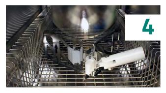
Place the opened frame lying on its side onto the sieve of the autoclave.
