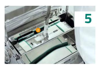
Activate the mop dosing unit in bucket 2 by pushing downward.
