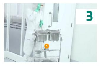
Open the mop frame by using the mop discard mechanism (pull upwards to unlock)
