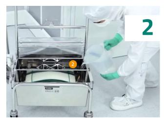
Fill in the needed amount of cleaning fluid in bucket 2, in which the mop dosing unit is placed.
