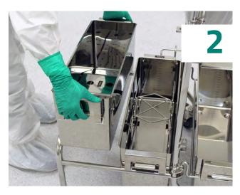
All removable components can be removed if necessary and added separately to the autoclave. All buckets must be autoclaved individually and without content.
