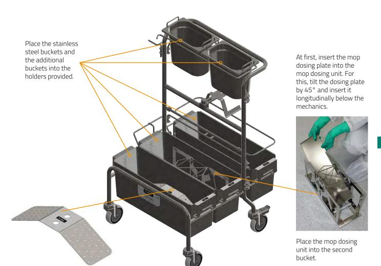
Insert the mop carrier into the front stainless steel bucket.
